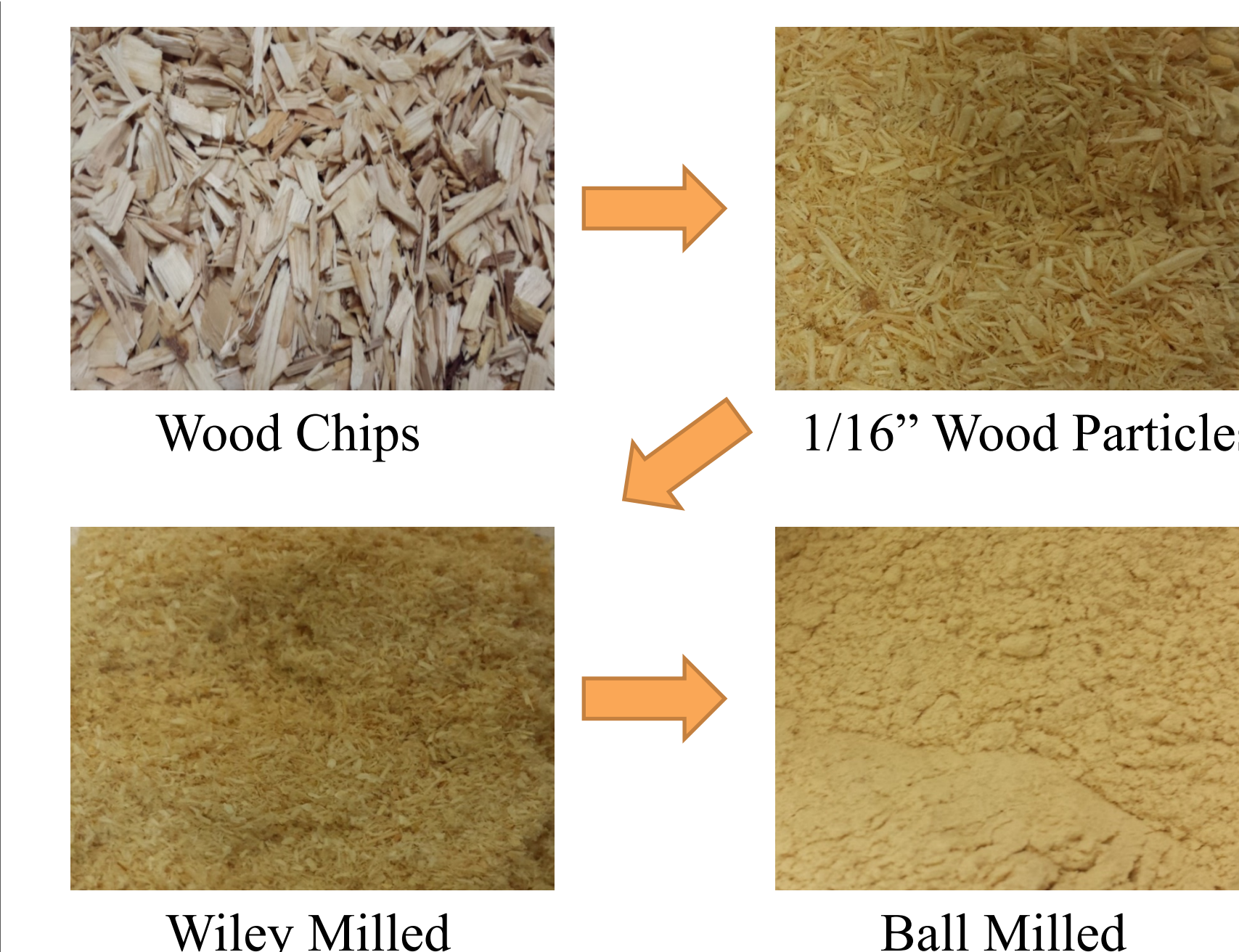
Fig. 3 Change of the size of the wood after 60 minutes of ball milling for the feed of 20 mesh. The total specific energy consumption was 21.9 MJ/kg wood, and the net energy used was 6.3 MJ/kg wood. D 10 means 10% volume cumulative distribution particle size.
