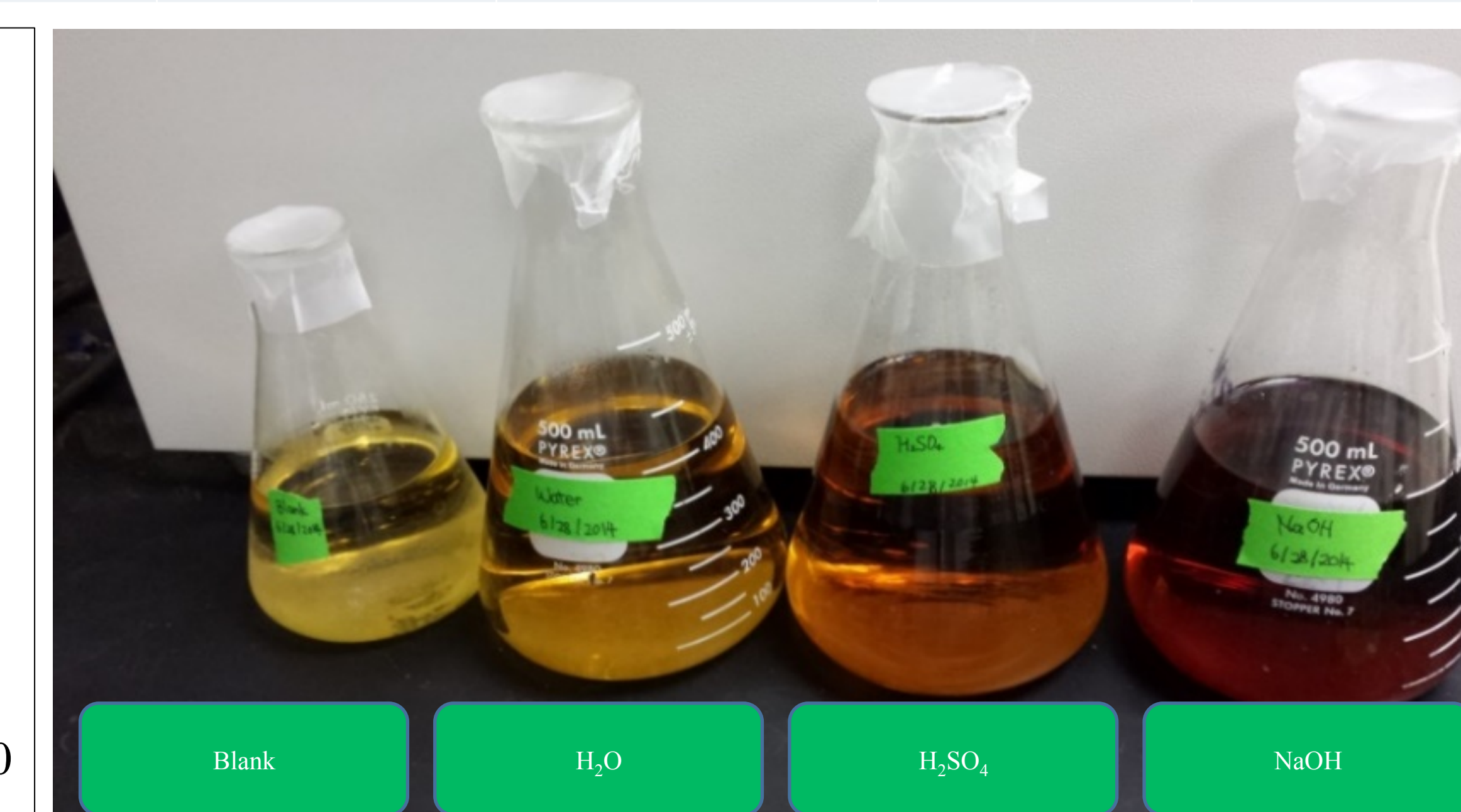
Fig. 5 Color difference of cellulosic sugars after enzymatic hydrolysis and filtration.
