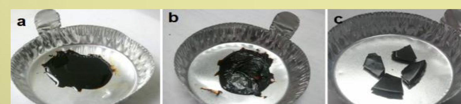
Visual state of PRFs without heat pretreatment (a) and after isothermal heat pretreatments of 60C (b) and 100C (c)
