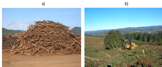
FIGURE 1.- a) Dry forest harvest residue, 15% MC; b) Green forest harvest residue, 60% MC
