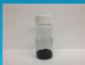
Figure 2: AC powder after carbonization, washing, and drying.
