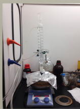
Figure 2: Reflux apparatus used to carry out demethylation.
