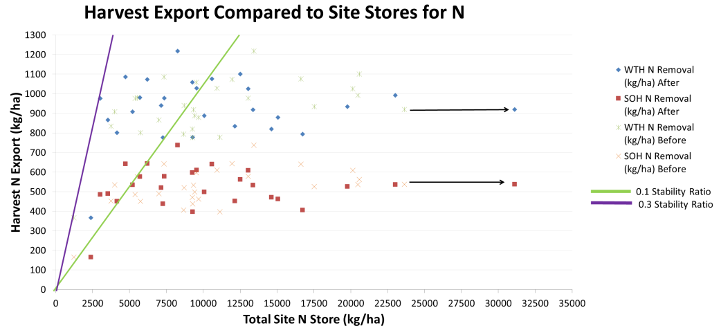
Figure 2. Above is a scatter plot where each point represents an extraction site and its relative distance from the stability ratio. Green asterisks' and orange X's represent the location of the points prior to this study while blue diamonds and red squares represent the location of the points after taking the new data into consideration. The green line represents a stability ratio of 10% nitrogen removal while the purple one represents a ratio of 30% nitrogen removal. 1 Points to the right of the green line represent sites that are not at risk of nutrient depletion and could potentially handle larger extraction rates. Points to the left of the purple represent sites that are at risk of depletion and require much more caution in terms of extraction. The results of this study show an overall shift to the right due to evidence of larger nitrogen stocks. Minor exceptions include points that were actually shifted to the left and can be attributed to the difference in pit locations and bulk density values between the two studies.
