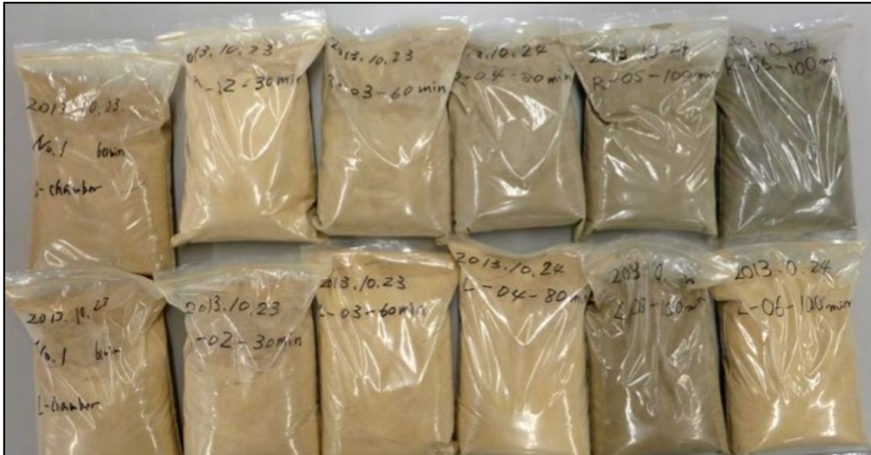
Figure SA-3. Milled wood powders of FS-10 chips, under various milling time, 30, 60, 80, and 100 minutes. Varying color of milled wood samples corresponds to milling temperatures. All materials were directly hydrolysable after milling with no chemical treatment.
