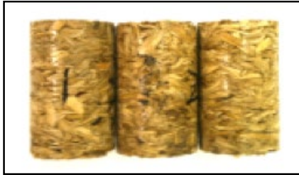
Figure E-8.1. Pellets consolidated with 12% MC, 150°C, 10 mesh, and 3% dextrin content
