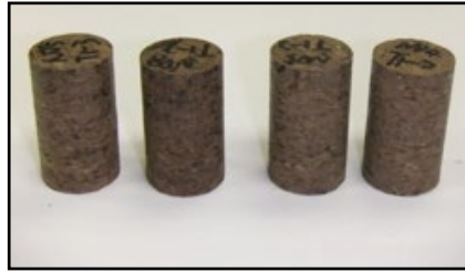
Figure E-8.2. Pellets densified with sodium sulfite treated particles under 160 oC for 10 min
