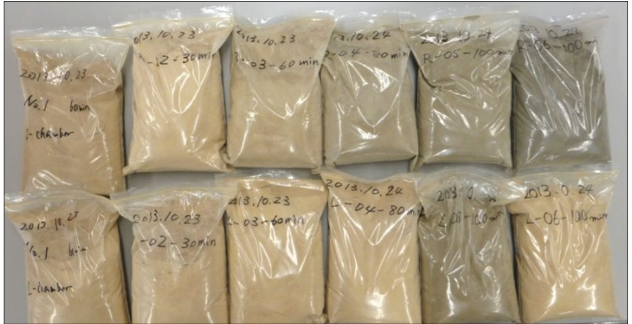
Figure C-P-5.6. Milled wood powders of FS-10 chips, under various milling time, 30, 60, 80, and 100 minutes. L-from left milling chamber; R- from right milling chamber. Lighter color of milled wood in L-chamber indicates milling temperature was cooler than that in the R-chamber (onsite photo during our visit to [redacted] )
