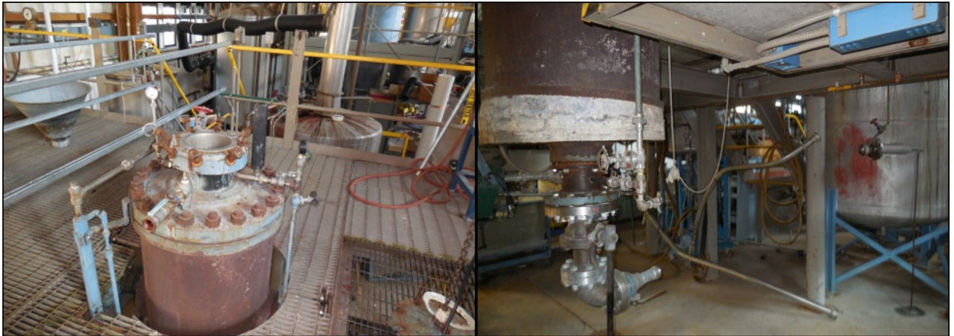
Figure C-P-1.3. The FPL pilot scale 390 L rotating reactor for pretreating 50 kg (oven dry) forest residue.
