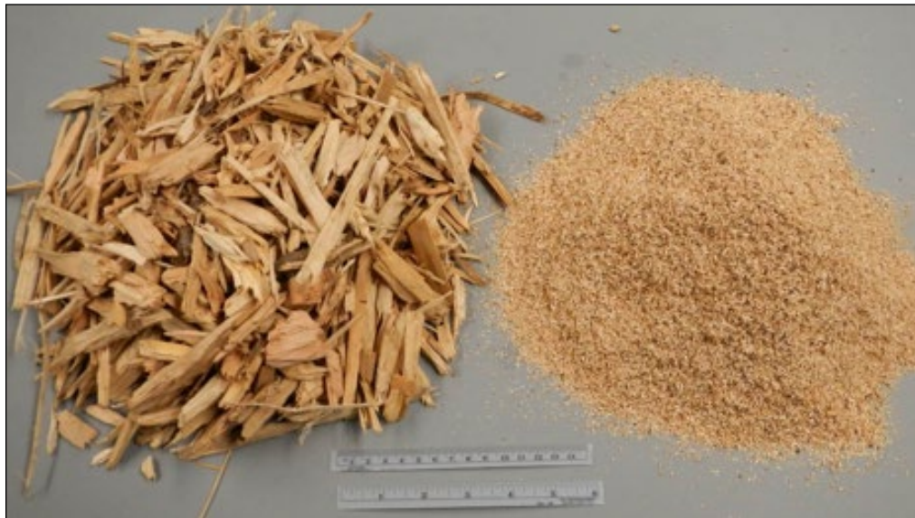
Figure C-P-5.1. Raw Douglas-fir FS-10 chips with 13.42 mm Xgm and finished feedstocks with 2 mm Xgm
