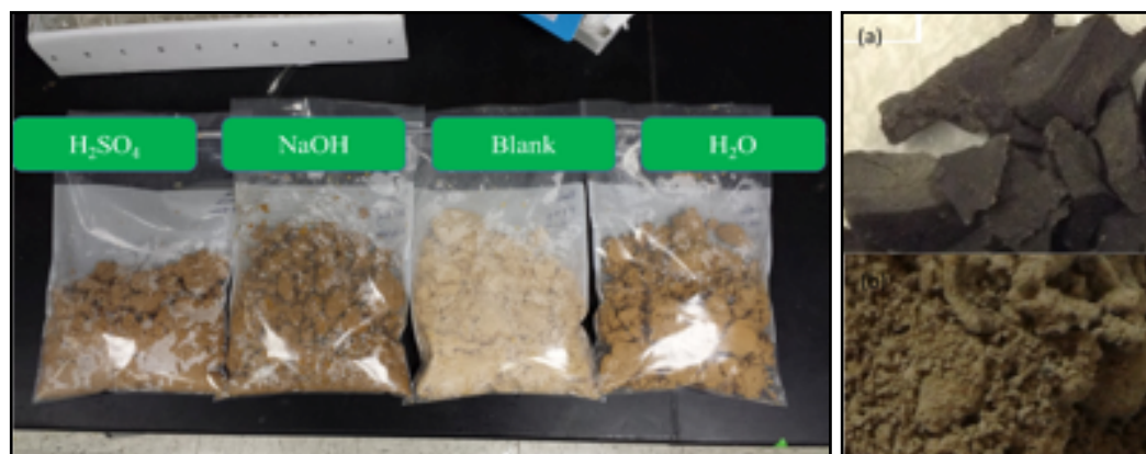
Figure E-8.5. Wet lignin residues after vacuum filtration. The color of the lignin residual without chemical treatments (Blank) is lighter. After dried at 103 °C overnight, it hardened into chunks (a) while other thermochemical treated residues looked like loose sandy materials (b).
