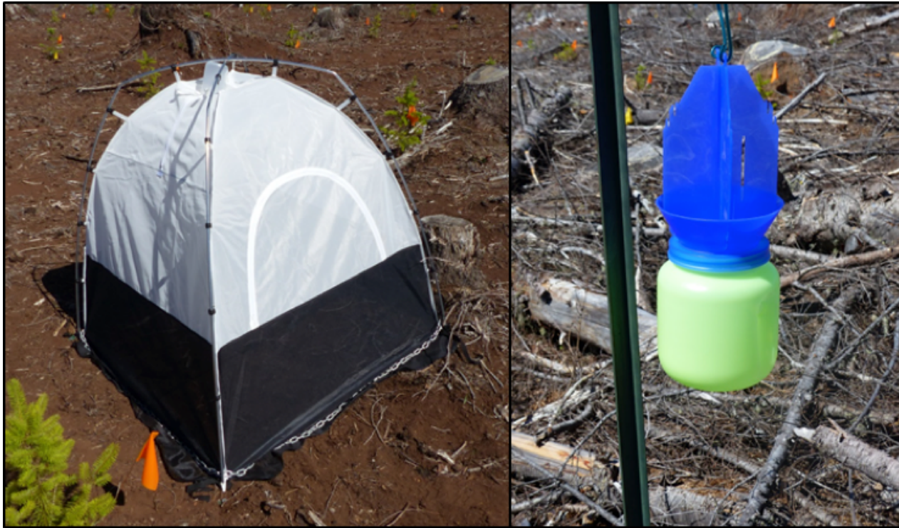
Figure SM-SP-6.1. Examples of a ground-nesting bee emergence trap (left) and a blue vane trap (right) used to trap invertebrate pollinators in the LTSP sites on Weyerhaeuser land during summer 2014. Emergence traps are enclosures with an open bottom that capture ground-nesting bees that overwinter in the soil and emerge as adults. In contrast, blue vane traps capture free-flying adult bees that vary widely in the type of substrates used for nesting.
