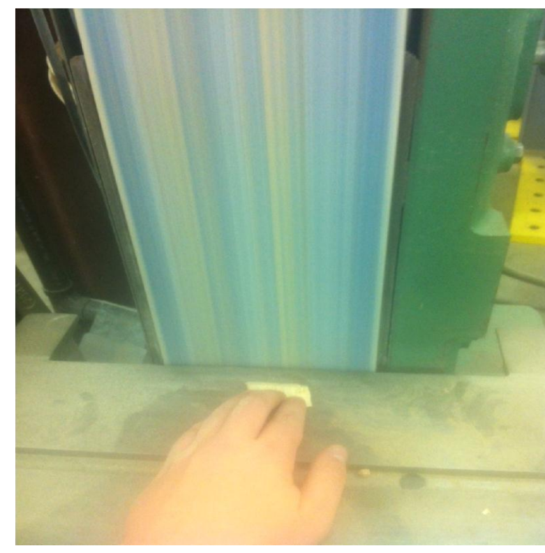
Step 1: Sand woodchip to a rectangular box shape
