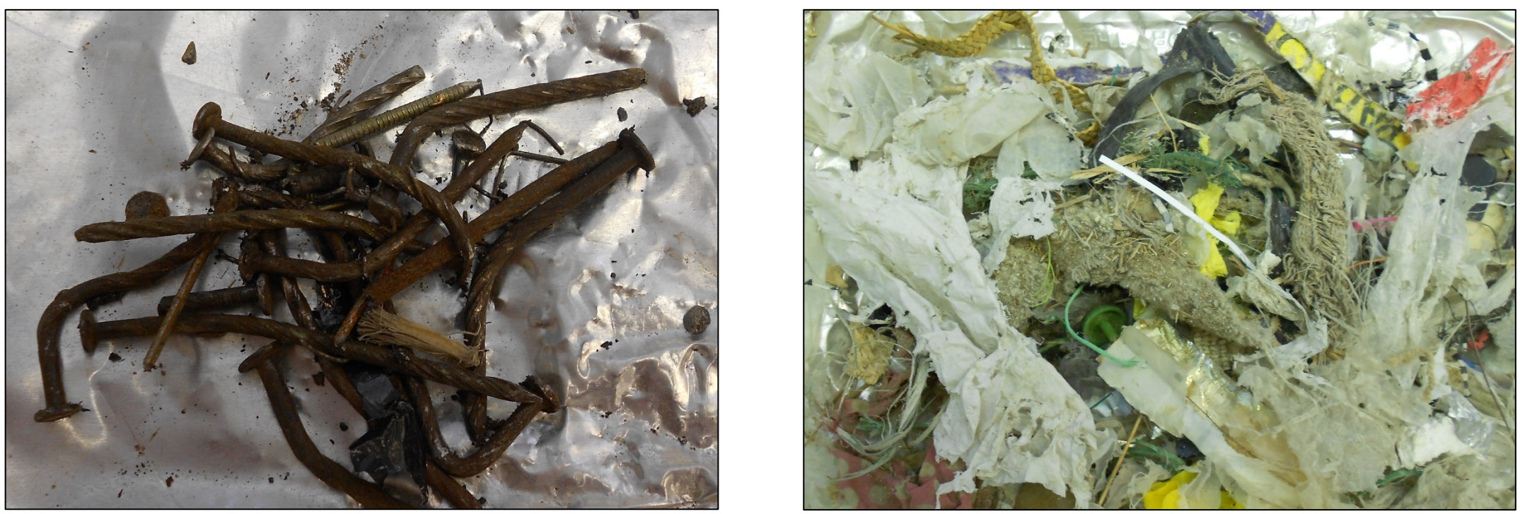
FIGURE 3 – Pictures of contaminants found in WWM samples: Metals (left) were found in sample 1 and other materials (e.g. plastics and fabrics) were found in sample 3.
