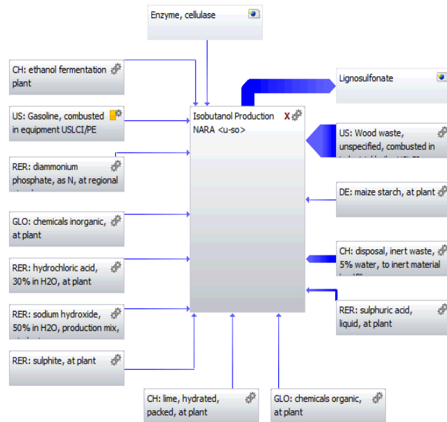
Figure 5. Initial structure of the isobutanol-to-fuel production pathway.
