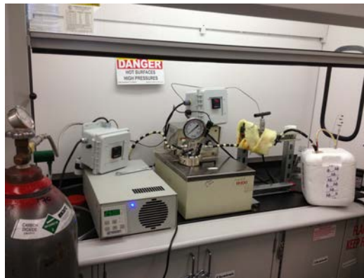
Figure 4: Supercritical carbon dioxide apparatus for extraction of platform molecules
