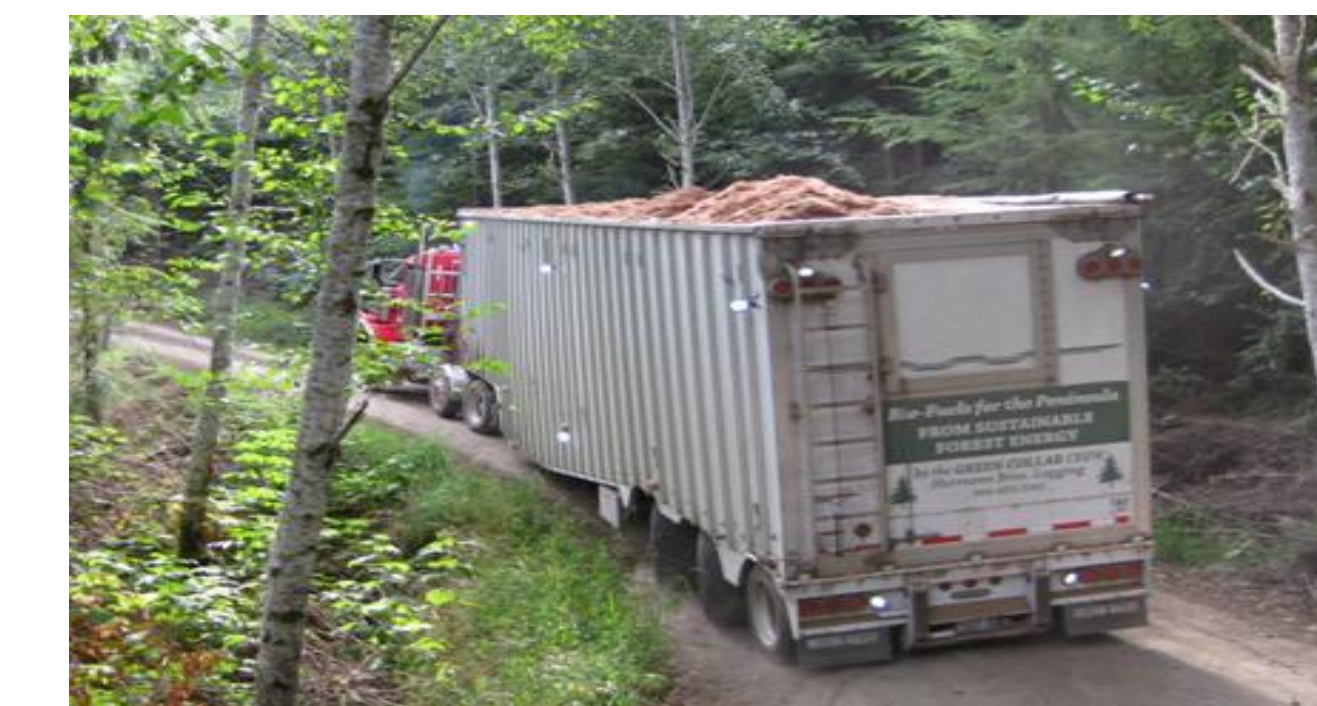
FIGURE 7. A 48-ft drop center trailer with self-steering trailer on a narrow forest road being pulled by 6x6 truck tractor.
