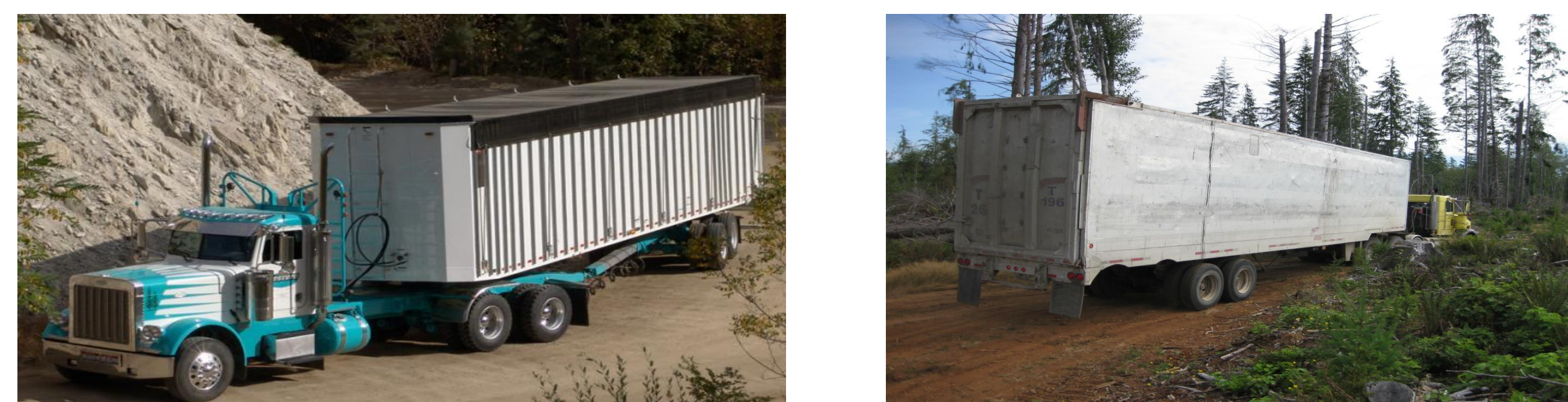
FIGURE 2. – A stinger-steered chip van (left) and sliding axle 5 th wheel chip van (right).
