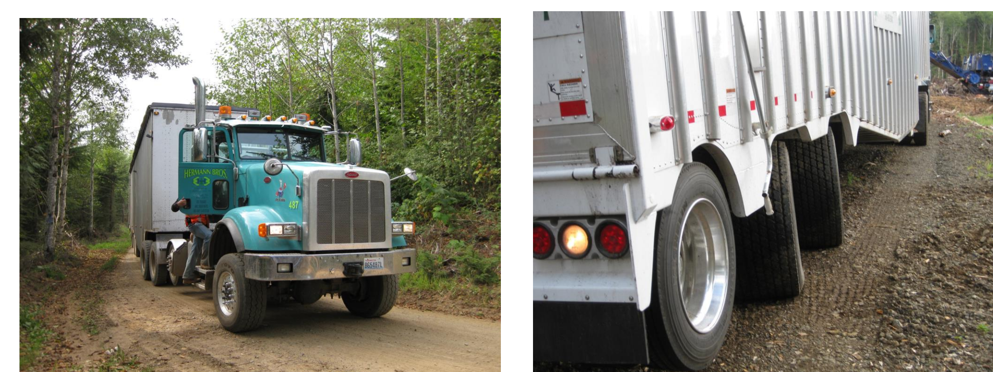
FIGURE 6. – A 6x6 truck tractor (left) and a self-steering trailer (right).
