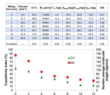
XRD and SEC reveal physicochemical structure destruction of milled wood cellulose.
