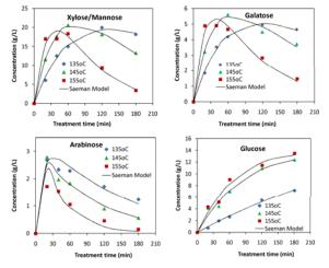
Obtain k1 and k2 with above data through Saeman model fitting for monomer sugars. Glucose didn't have a complete hydrolysis and degradation curve during 3 hours cooking.
