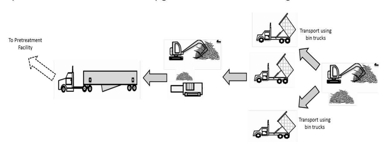
System 2. Bundled at the site without grinding (processed with electric grinder at facility)
