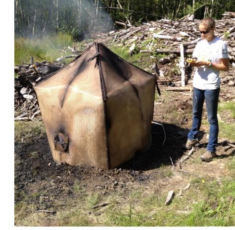
and portable method to process biomass that has in the past gone to waste. This new technology uses a thermal insulating material that captures and evenly distributes heat released from the partially combusting pile.
