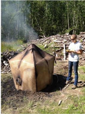
Our thermal processing unit was developed to create an economical and portable method to process biomass that has in the past gone to waste. This new technology uses a thermal insulating material that captures and evenly distributes heat released from the partially combusting pile.
