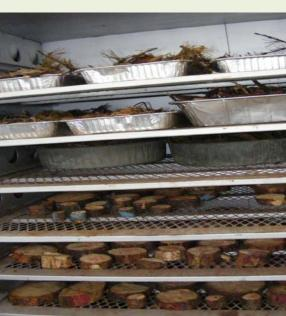
Each sample was weighed before being put in the oven at 103° Celsius. The tins are filled with samples from ground piles, and the bottom half of the picture are samples from pre-ground piles. Each sample was put in the oven for 48 hours and then was weighed again.
