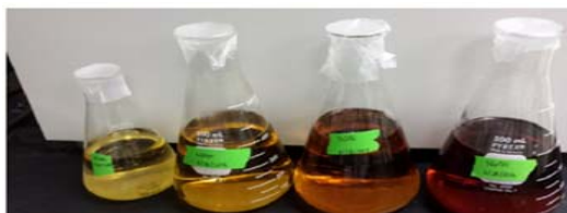
Fig. 6 Color difference of clarified enzymatic hydrolyzates. The light color of the hydrolyzate from the mechanical pretreatment indicated its less inhibitors, confirmed by smaller intensity at 280 nm (furfurals) and by the HPLC analysis.
