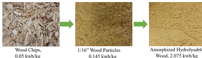
Fig. 2 Total actual milling energy of 2.27 kwh/kg is based on a pilot scale system. The result is strong and sets us up for success at scale up. The larger machine is expected to be more energy efficient. So does that justify the 2015 funding because we are well in reach to proceed to a larger scale processing to achieve overall goal of 1.5 kwh/kg.
