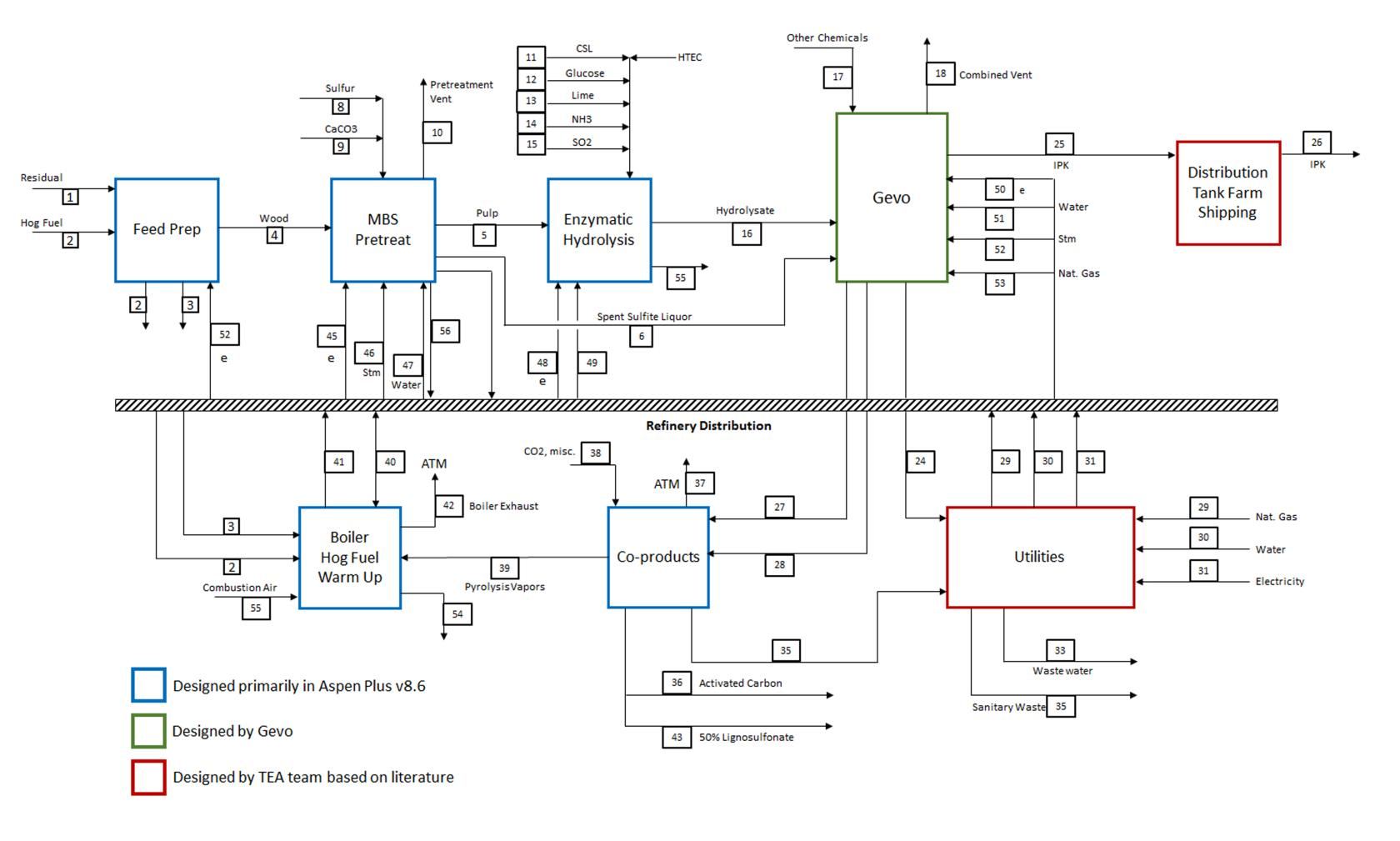
Figure: Nara integrated biorefinery model. Streams represent mass and energy balances calculated with Aspen and from literature analysis.
