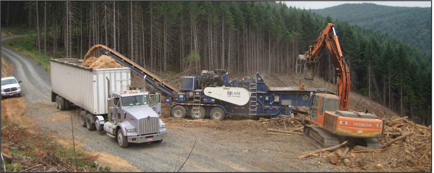
On-site grinding of forest residuals. Photo from John Sessions, Oregon State University
