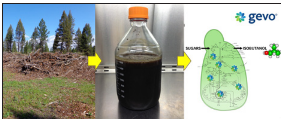
Conversion process from forest residuals to hydrolysate to isobutanol. Images courtesy of Gevo, Inc
