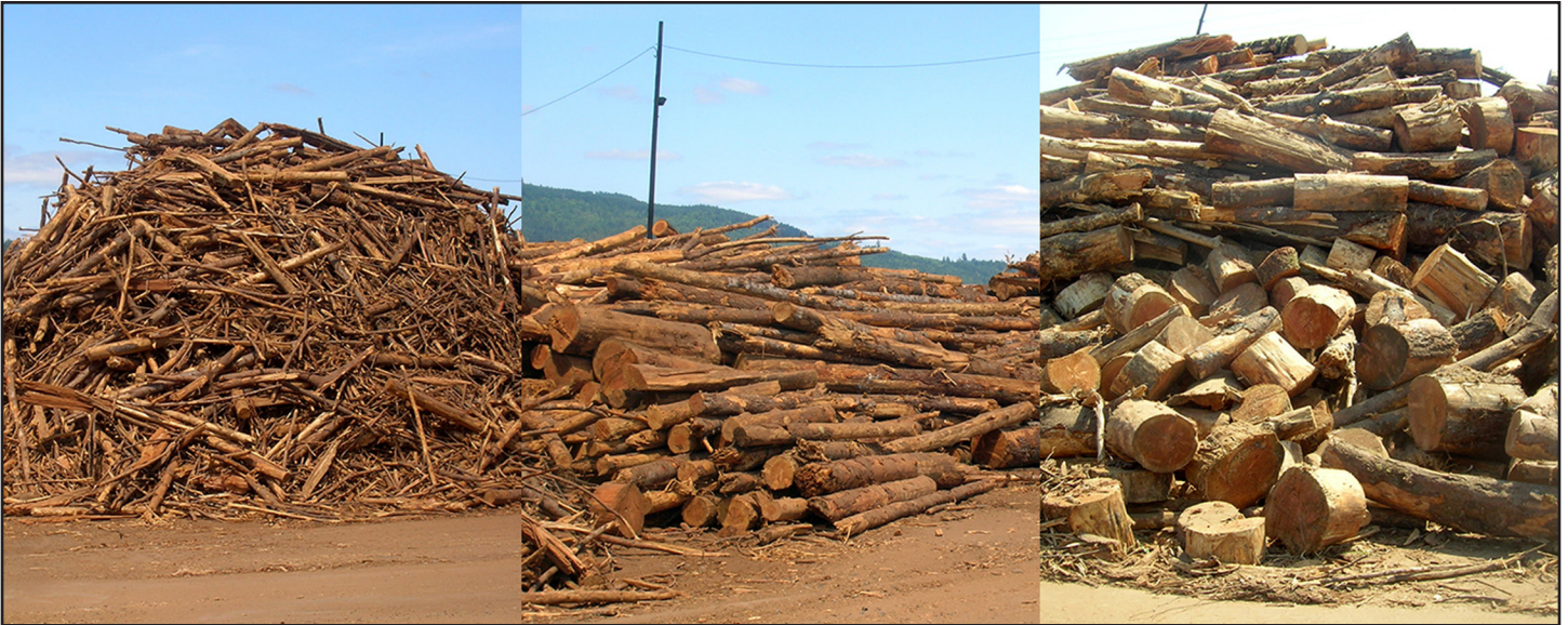
Forest residuals used in grinding tests. From left to right: branches and tops, pulpwood, butt-log-chunks. Images courtesy of Rene Zamora-Cristales, Oregon State University.
