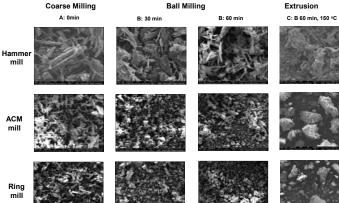
SEM micrographs reveal fiber delamination and cellular fragmentation of pretreated Douglas-fir
