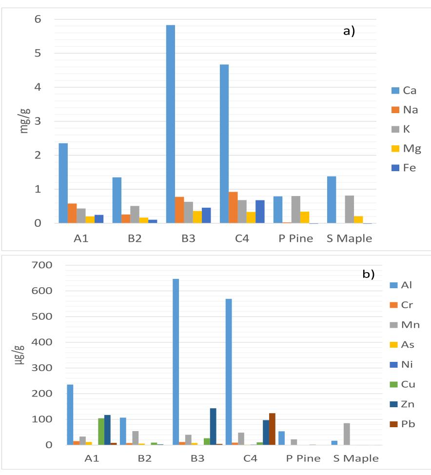
ICP-MS results showing content of alkalines and metals in the WWR samples (as received). Ponderosa pine and sugar maple have been added for comparison purposes only.
