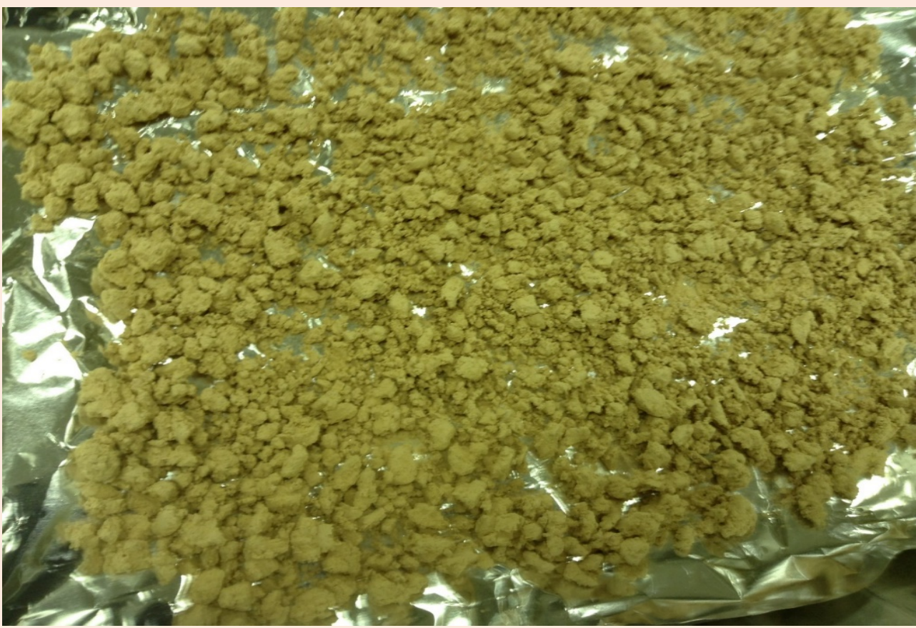
Fig. 2 dry lignin residues. moisture is around 5%
