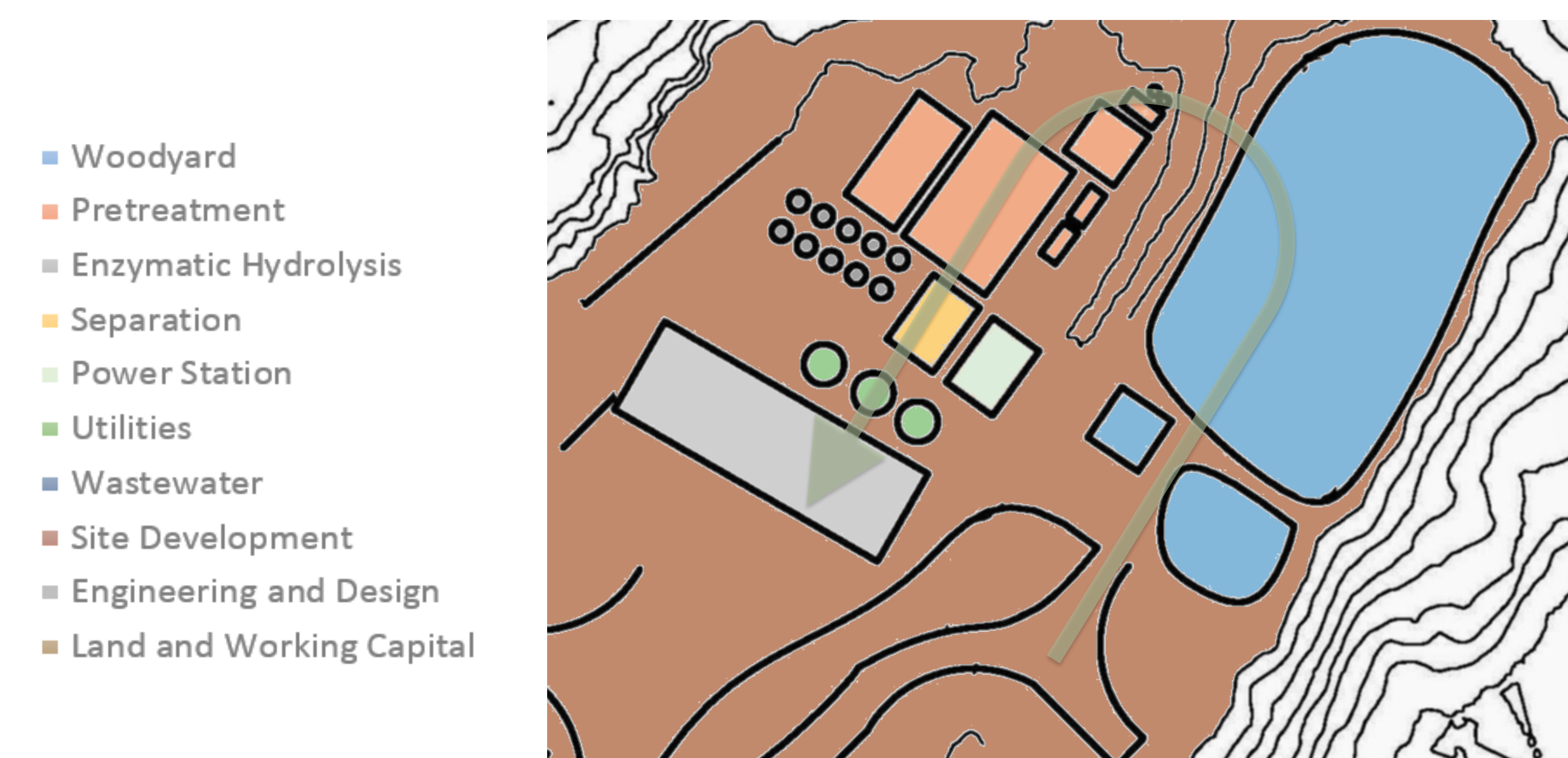
Figure 3: Proposed site design for a liquids depot. The map is to scale with the areas colored according to the charts shown in the right column. The flow through the facility is represented by the green arrow.
