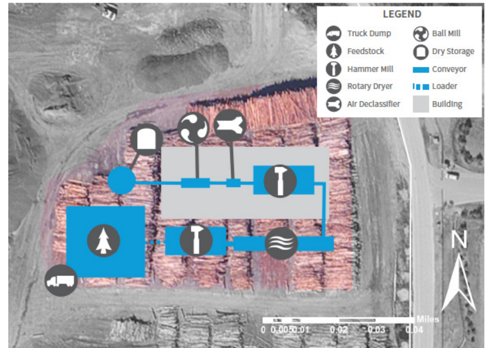
Figure 2.3.12 Hermann Brothers Site A Equipment Layout
