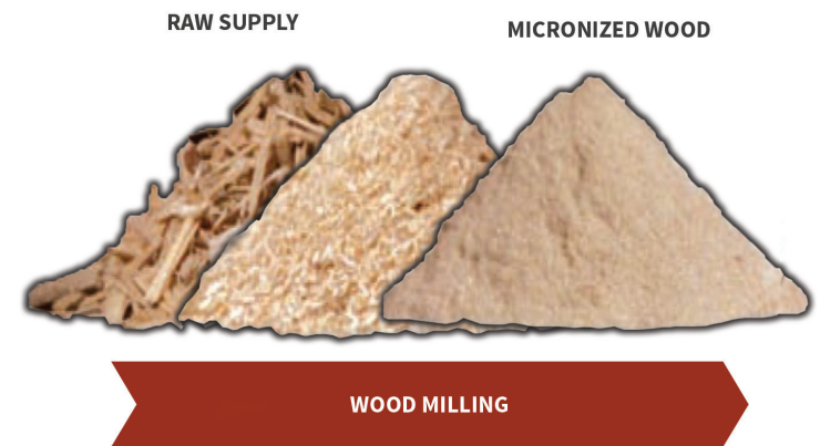
Figure 2.3.3 Transition of Forest Residuals from Chips to Flour
