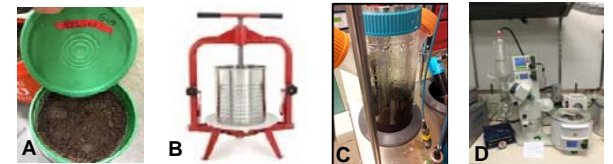
Figure 6. Hydrolyzed material as received from Andritz FS-20 trial (A) and processing steps at Gevo. (B) Fruit and wine press used to press as-received solids, which were also washed with 1 volume of water equal to the pretaste. (C) DasGip 2L vessel filled with 3 marine style impellers and electrically-controlled heating block used to perform enzymatic saccharification. (D) 1L nominal volume RotoVap rotary evaporator used to concentrate hydrolyzate up to sugar levels of ~150 g/L.
