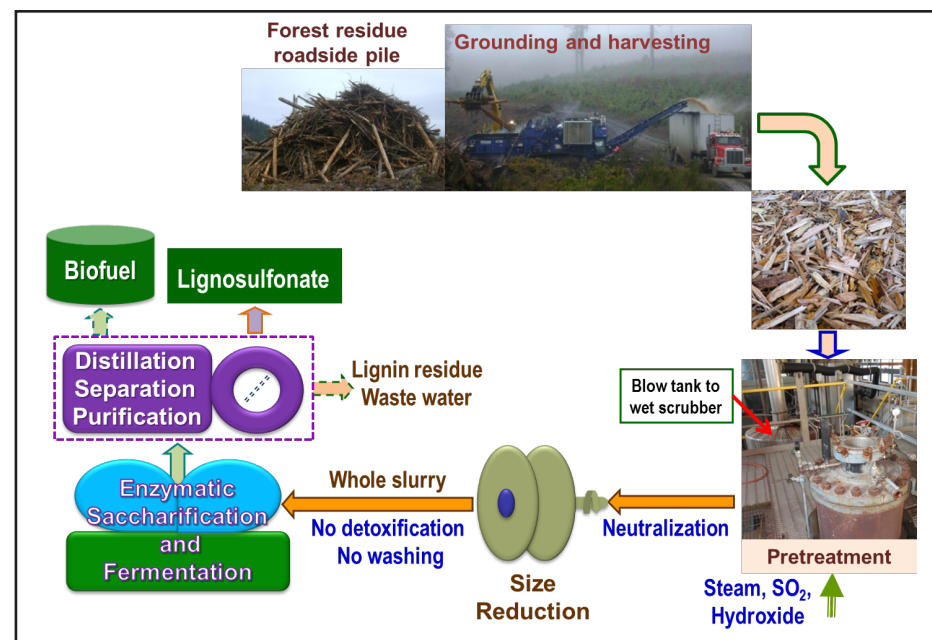
Figure SP-2.1. A schematic process flow diagram shows Douglas-fir forest residue harvesting, transportation, pretreatment and downstream saccharification and fermentation.
