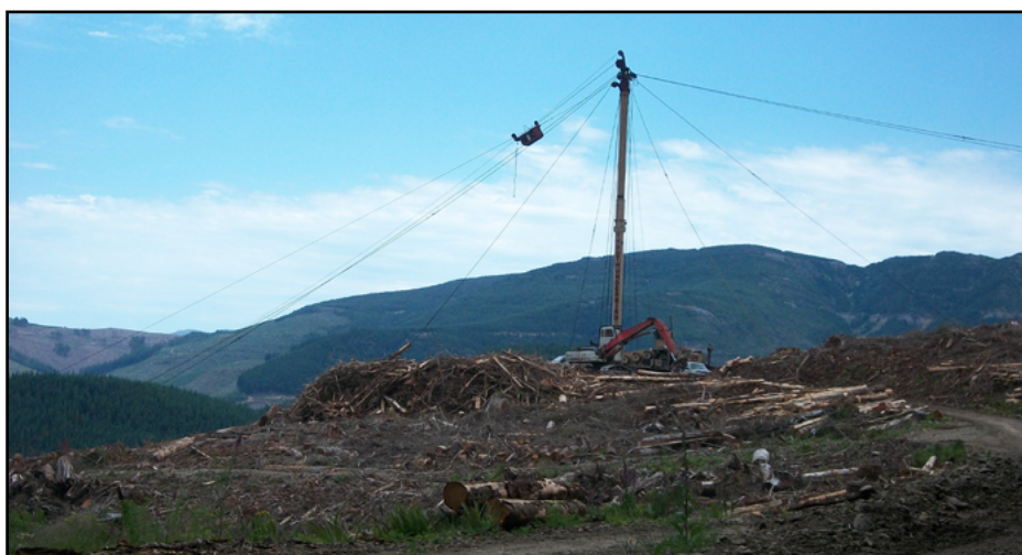
Figure TPO-3.4. Skyline yarder with radio-controlled carriage (Photo by Eric Simmons, BBER).
