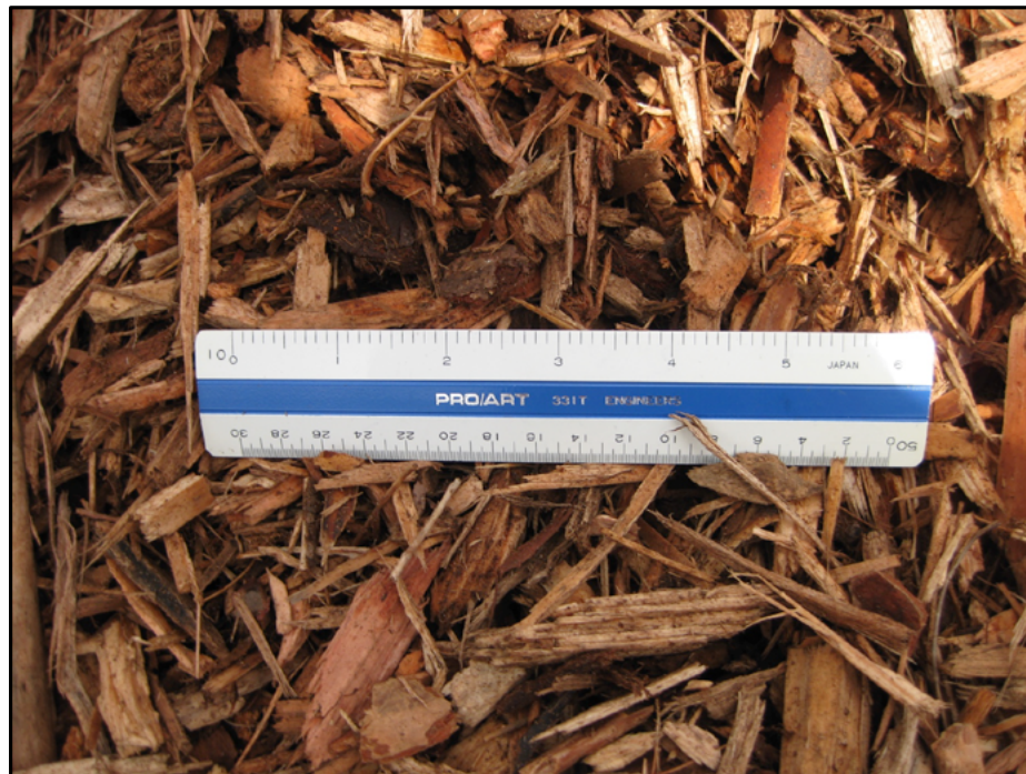
Figure FS2-A2.4. FS-17 first pass screen accepts (-1"WW, +1/8" WW) FS-17, about 75% of feed.
