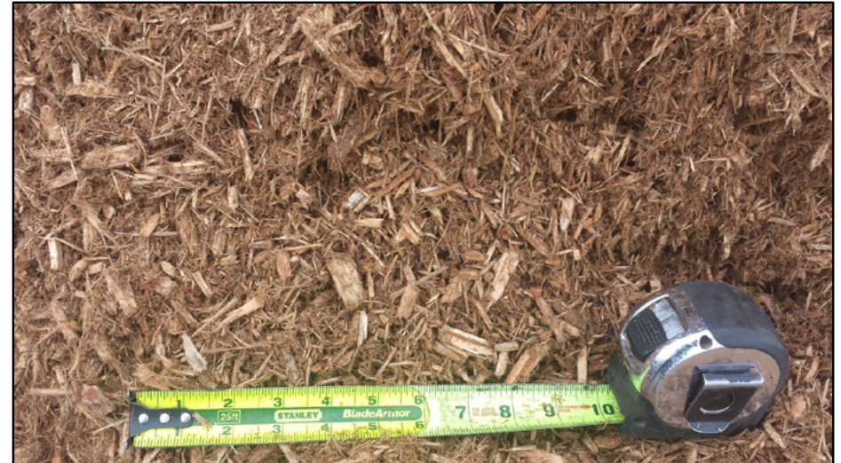
Figure FS2-A2.10. FS-20C test grind through horizontal grinder B-1-1-1.5 grates.
