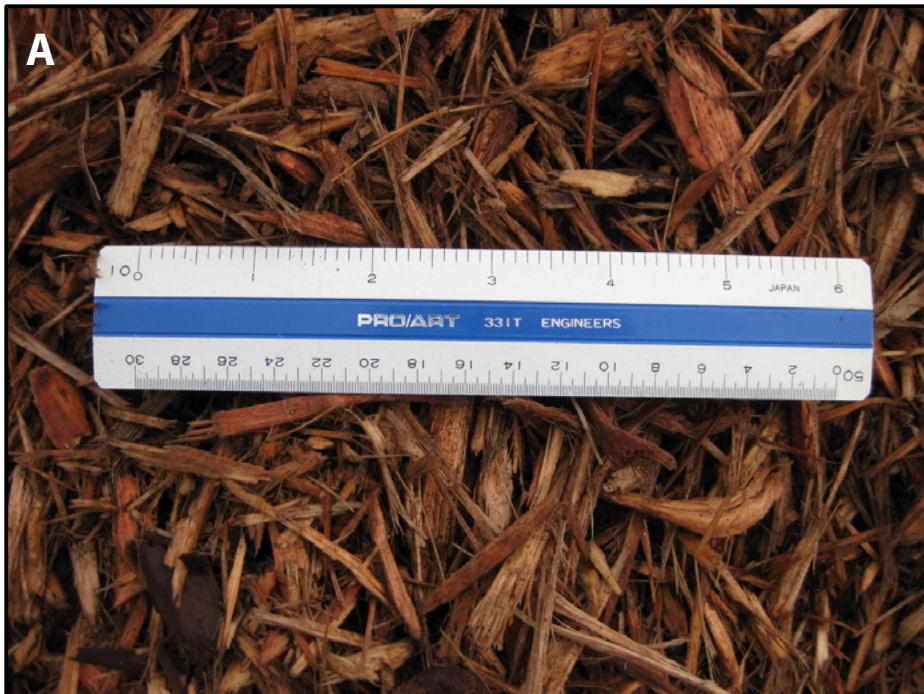
Figure FS2-A2.6. Three FS-17 feedstock sizes: Oversize in foreground, Accepts in mid-shot, and Fines in the background.
