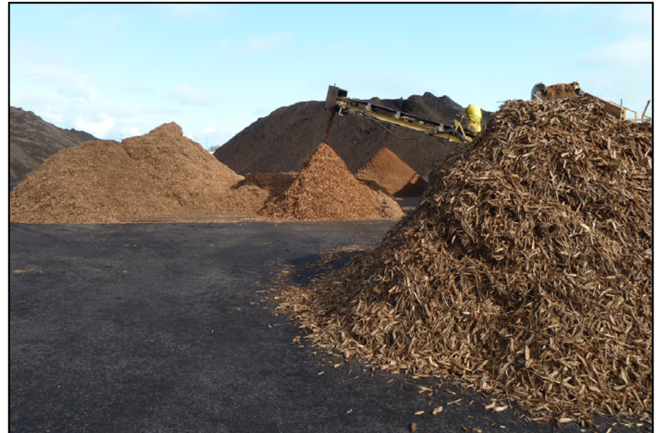
Figure FS2-A2.6. Three FS-17 feedstock sizes: Oversize in foreground, Accepts in mid-shot, and Fines in the background.
