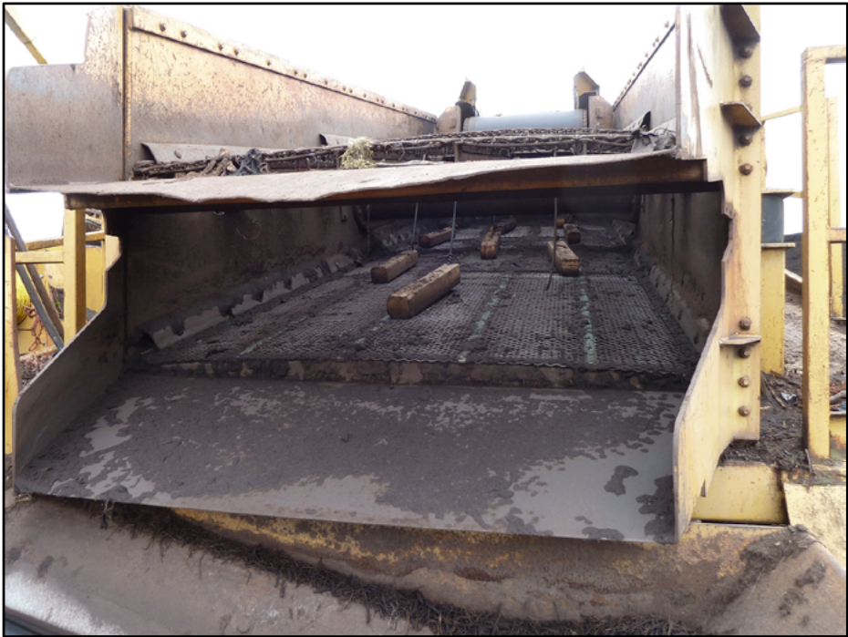
Figure FS2-A2.2. Screening system at Lane Forest Products
