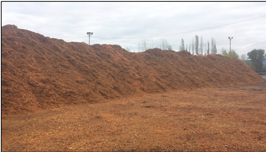
Figure FS2-A2.9. FS-17 Accepts and re-ground overs with 5% Washington and Montana Accepts added, ready to blend and re-size.
