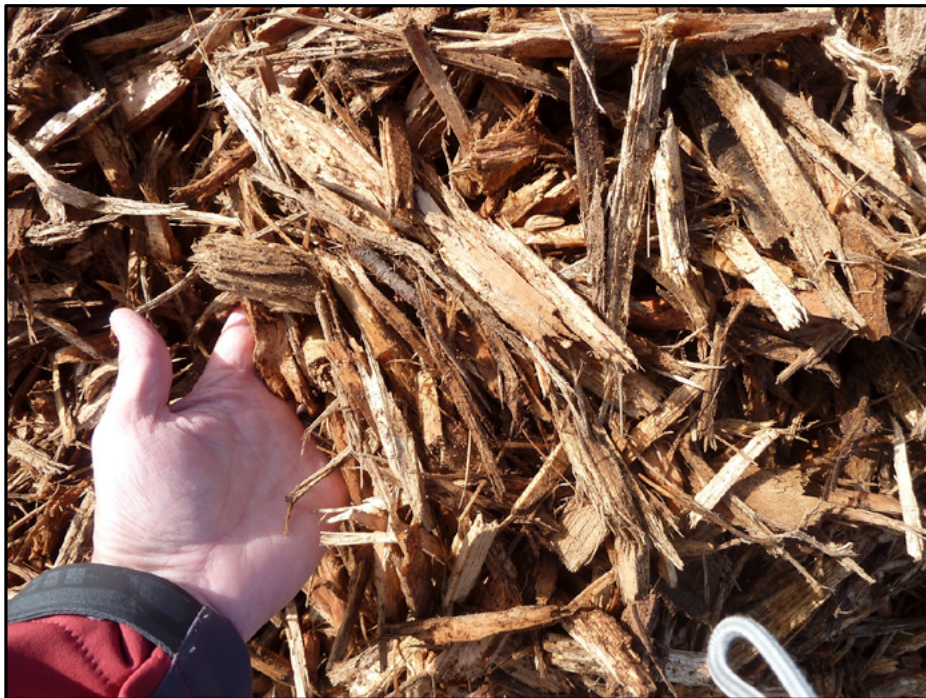
Figure FS2-A2.3. Oversized FS-17 screened with 1" woven-wire top deck. About 15% mass rejected.
