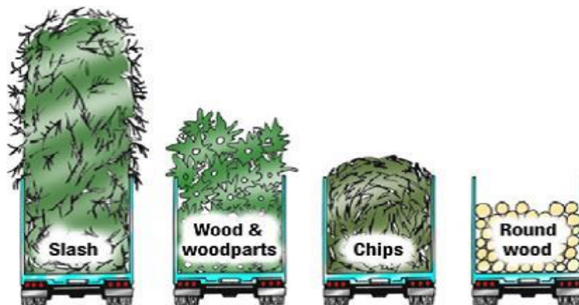
Figure 3. Volume Differences of the same Weight Material by Different Product Types ( http://www.extension.org/pages/70315/biomass-transportation-and-delivery#.VTq5mWRVikp )
