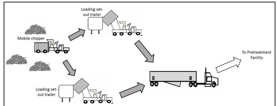
Figure LCA-1.3. System 3: Mobile chipper with set-out trailer. Logging truck with trailers is used for hauling.
