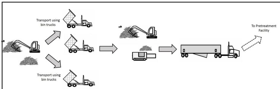
Figure LCA-1.1. System 1: Bin truck with stationary grinder at centralized landing. Chip van is used for hauling processed residues.
