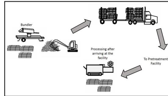
Figure LCA-1.2. System 2: Bundling in forest and processed with electric grinder at facility. Bundles are processed with electric grinder at the facility.
