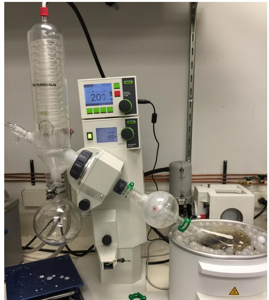
Figure LIF-5.9. RotoVap setup used to concentrate sugars in low solids hydrolyzate.
