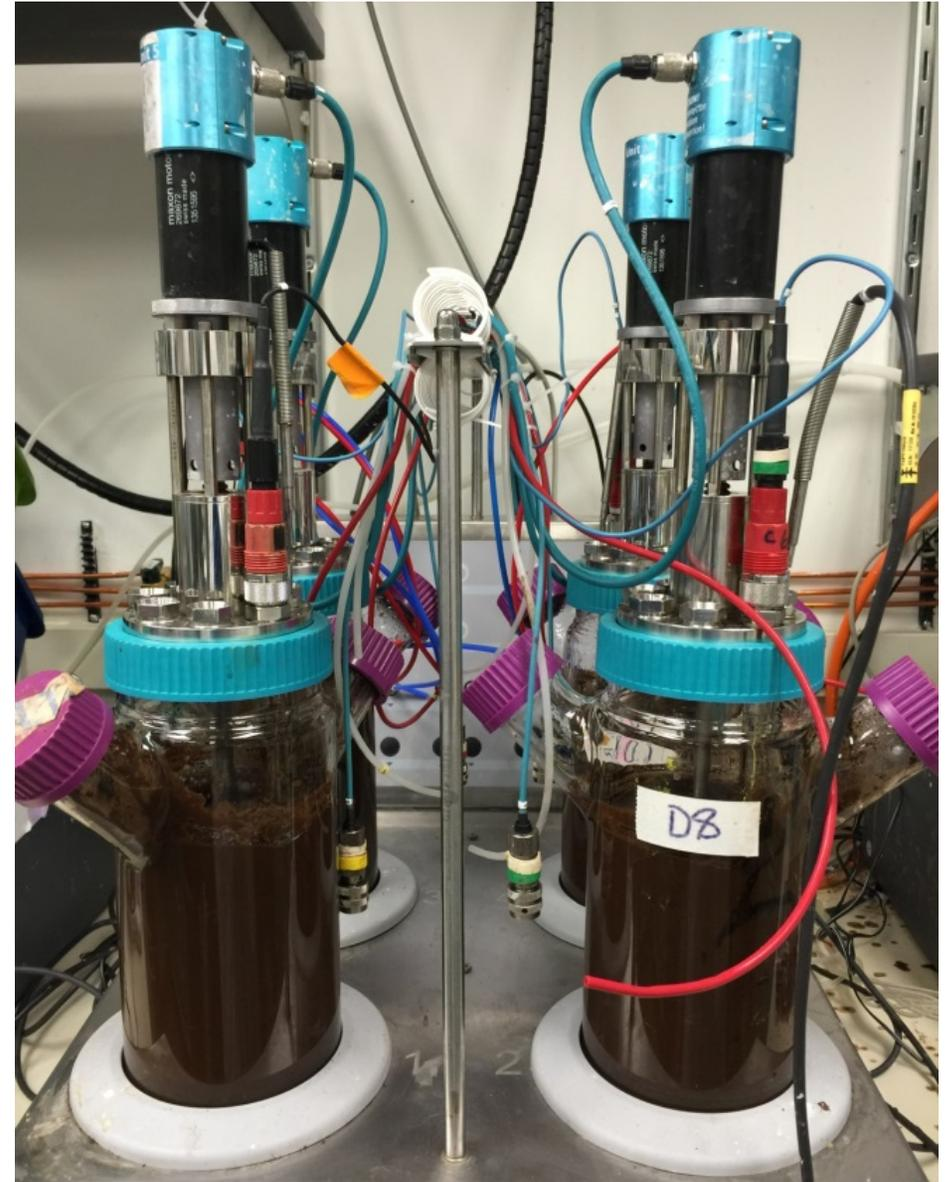
Figure LIF-1.18. 2L nominal volume DasGip bench-scale fermenters used for hydrolysis. The fermenters have top-drive motors with agator shafts fitted with three marine-style impellers for superior mixing during hydrolysis.
