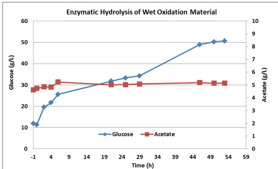
Figure LIF-1.2. Enzymatic hydrolysis test for 24% wet oxidation pretreated biomass. Hydrolysis was done in a pH-controlled 2L fermentor (pH5) at 50°C. Addition of 0.1 ml CTec2 (Novozymes) per gram glucan at 0 hours and 24 hours.
