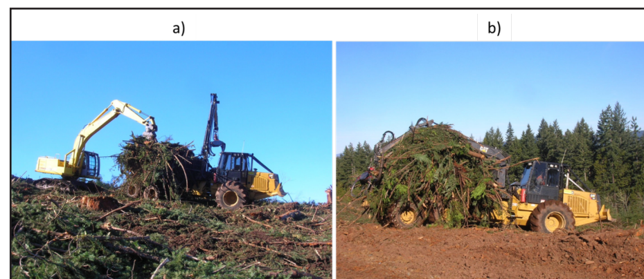
Figure FL-3.5. a) Forwarder being loaded by the excavator-base loader; b) Forwarder traveling to the landing.
