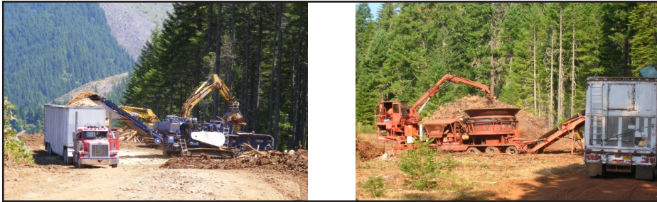
Figure FL-3.11. Stationary grinders performing in-field processing operations. Horizontal grinder (left) processing residues near Springfield, Oregon USA. Tub Grinder (right) processing residues near Medford, Oregon, USA.
