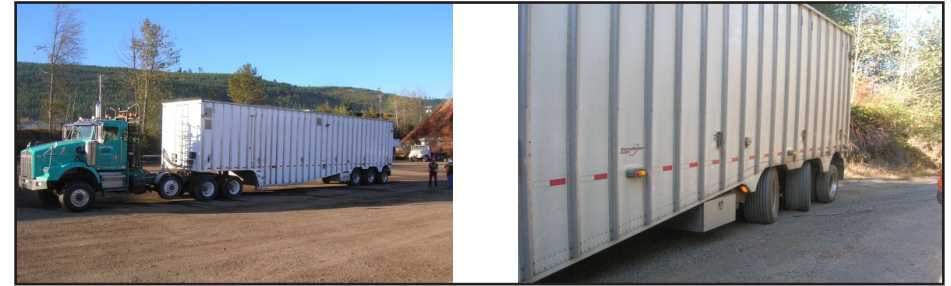
Figure FL-3.15. Rear-steer axle chip trailer operating in Port Angeles, Washington. This configuration is comprised of a tri-axle trailer (left) with two steering axles (right).
