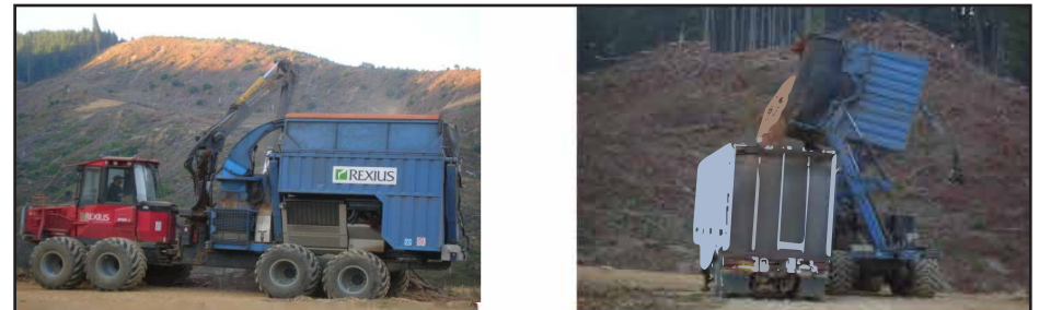
Figure FL-3.10. Mobile chipper processing forest residues near Elkton, Oregon, USA. Processing a road-side pile (left); unloading a bin of chips into a set-out trailer.
