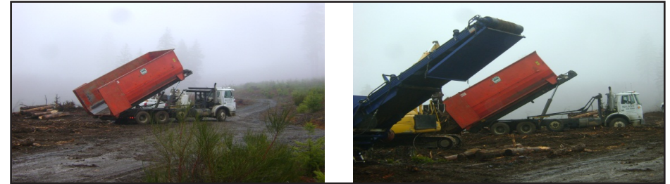
Figure FL-3.12. Hook-lift trucks in biomass recovery operations near Eugene, Oregon, USA. The trucks were transporting residues to a centralized landing where a stationary grinder was located.
