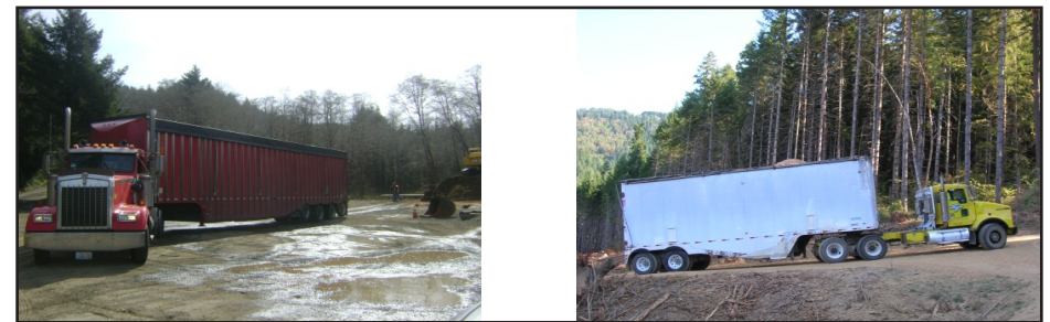
Figure FL-3.13. Chip vans hauling processed forest residues. A 6x4 truck hauling a 16.5 m long drop center trailer in Rockaway, Oregon, USA (left). A 6x4 truck hauling a 9.75 m drop center trailer in Elkton, Oregon, USA (right).
