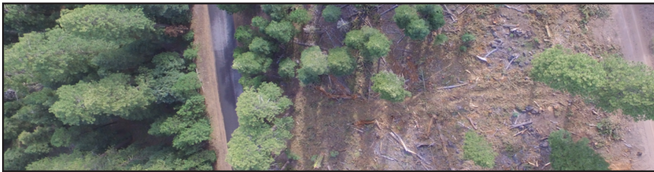
Figure FL-3.E.5. Reconstructed image using structure from motion to develop photogrammetric point cloud and xyz coordinates at 3 cm pixel resolution.
