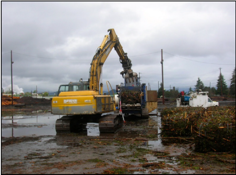
Figure FL-4.31. Loading bales tangentially into grinder at International Paper site, Springfield, OR.
