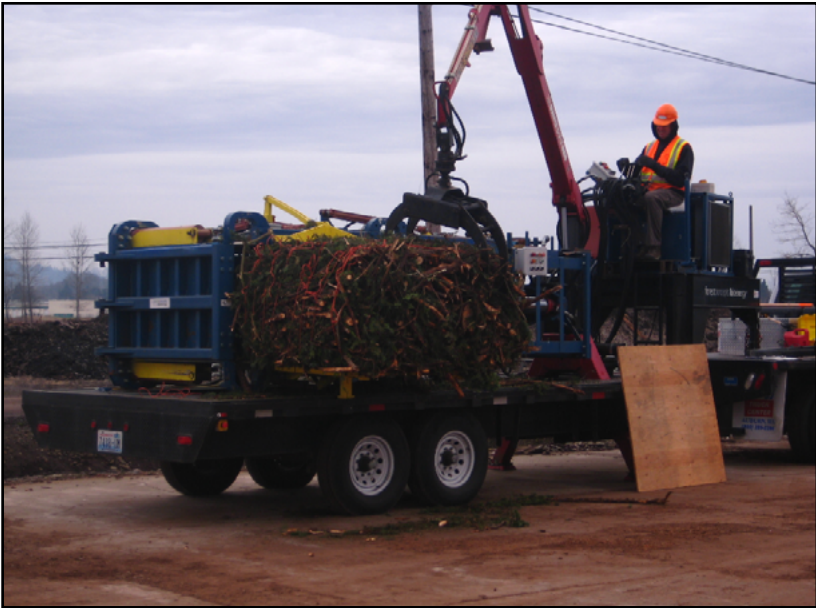
Figure FL-4.30. Producing bales utilizing a small baler provided by Forest Concepts.
