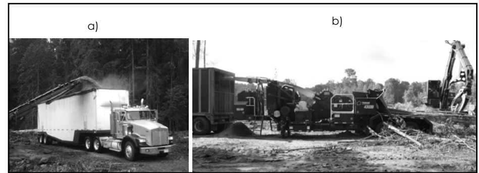
Figure FL-4.11. a) Conveyor-fed loading method into a chip van in a grinding operation; b) Horizontal blowing of wood chips into trailers.
