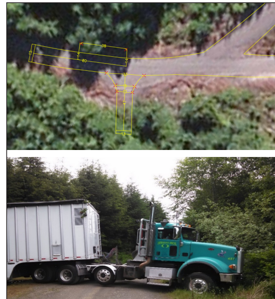
Figure FL-5.11. In a multi-part turn, the truck backed into a 47-ft deep stub, 13-ft wide with a 32-ft throat. At points during the turn, the back of the trailer was off road, as well as the truck-tractor was forward into the ditch.
