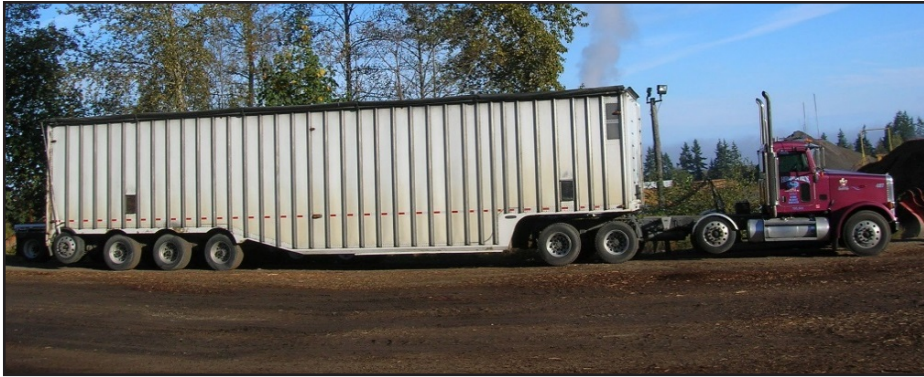
Figure FL-5.33. A 16.2m drop center 5th-wheel chip van near Port Angeles, Washington.
