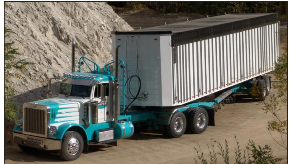
Figure FL-5.32. A stinger-steered chip van. Photo courtesy of Western Trailer Company.
