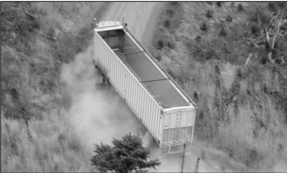
Figure FL-5.1. Truck Tractor with 5th wheel chip van on a horizontal curve. Reed's Fuel & Trucking operating near Dillard, OR.
