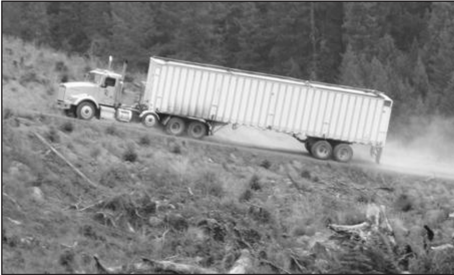
Figure FL-5.8. Truck tractor with unloaded chip van on 15% adverse grade. Sliding trailer axles in forward position. Reed's Fuel & Trucking operating near Dillard, OR.
