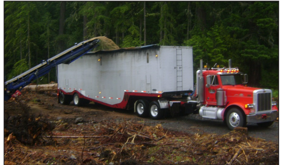
Figure FL-5.31. A 13.7m drop center 5 th -wheel chip van being loaded on a forest road in Lane County, Oregon.
