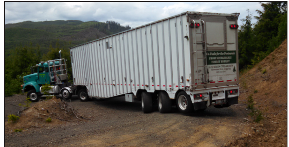
Figure FL-5.14. Negotiating a 180-degree switchback. Note direction of trailer tires.
