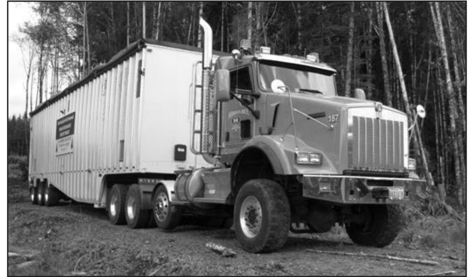
Figure FL-5.7. All-wheel drive truck tractor with 5th wheel chip van with steerable rear axles. (Hermann Brothers, Port Angeles, WA).
