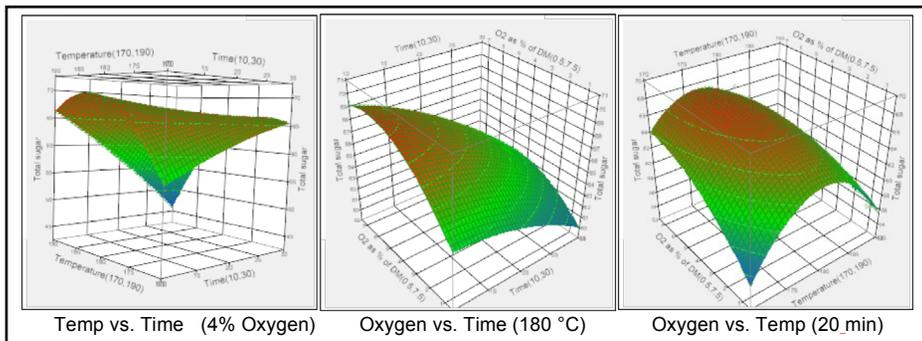
Figure PPB-7. Factors effect on FS-10 pretreatment for total sugar extraction in the liquid fraction of pre-treated slurry.
