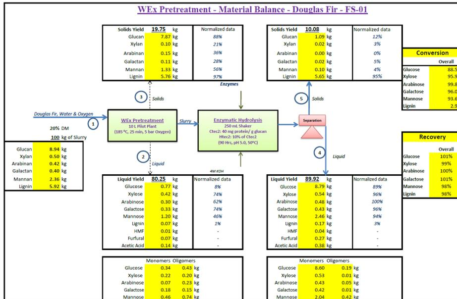
Figure PPB-3. Mass balance of FS-01 sample under optimized process conditions.
