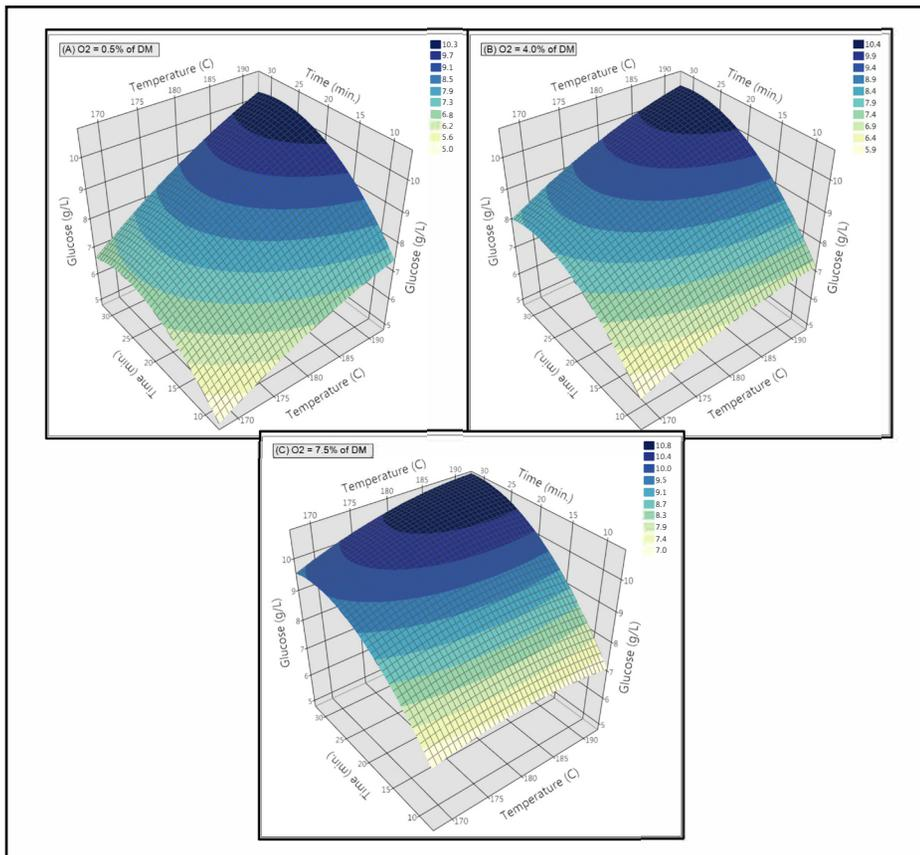
Figure PPB-5. Response surface models for glucose concentration after 72 hours of enzymatic hydrolysis (at pH 5.0, solids concentration of 10%, enzyme loadings of 40 mg EP/g glucan) of the pretreated samples at different oxygen loading (% w/w); (A) Oxygen loading of 0.5% of DM, (B) Oxygen loading of 4.0% of DM, (C) Oxygen loading of 7.5% of DM.
