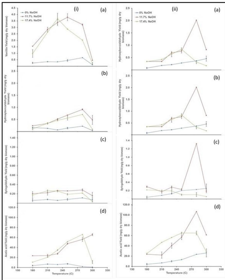
Figure PPB-app.3. Variation in concentration (mg/g dry biomass) of lignin oxidation products (a) vanillin, (b) hydroxybenzaldehyde, (c) syringaldehyde, and (d) acetic acid as a function of temperature at different NaOH loadings and residence time of (i) 5 mins and (ii) 15 mins. (● – 0wt% NaOH; ▲ – 11.7wt% NaOH; ■ – 17.4wt% NaOH)
