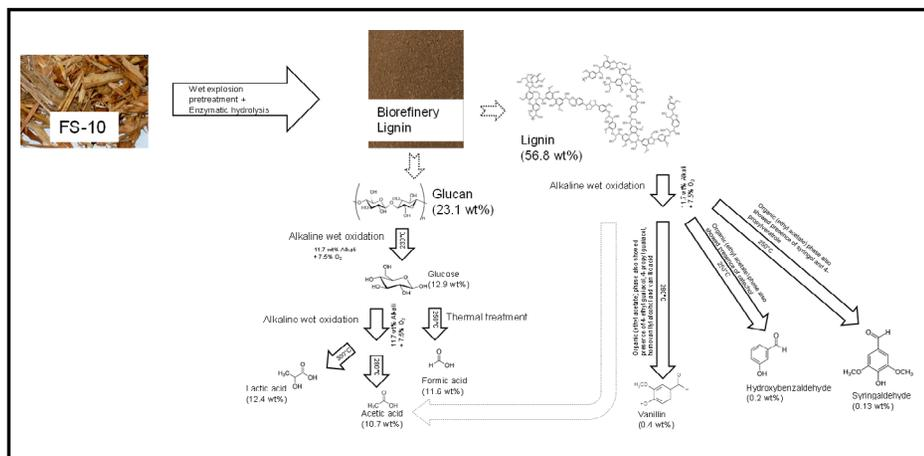
Figure PPB-app.4. Overall process reaction scheme showing the alkaline wet oxidation of biorefinery lignin to bioproducts.
