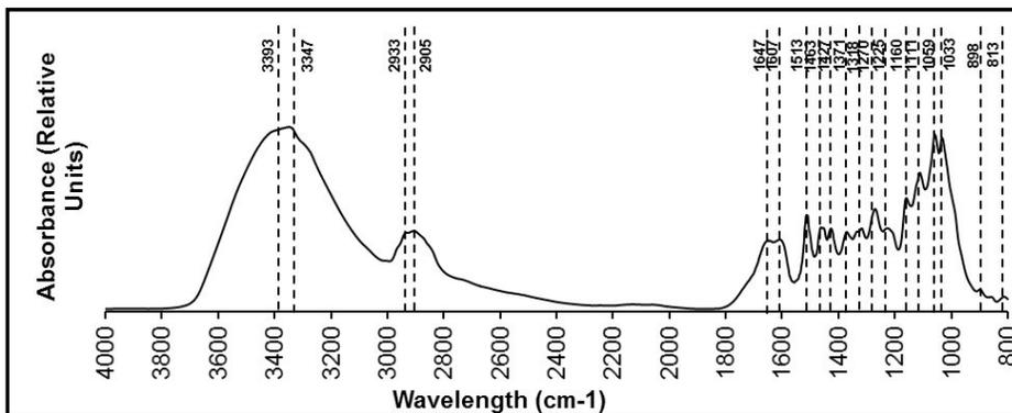
Figure PPB.app.2. FTIR spectra of biorefinery lignin stream showing spectral bands pertaining to component peaks present in biomass.
