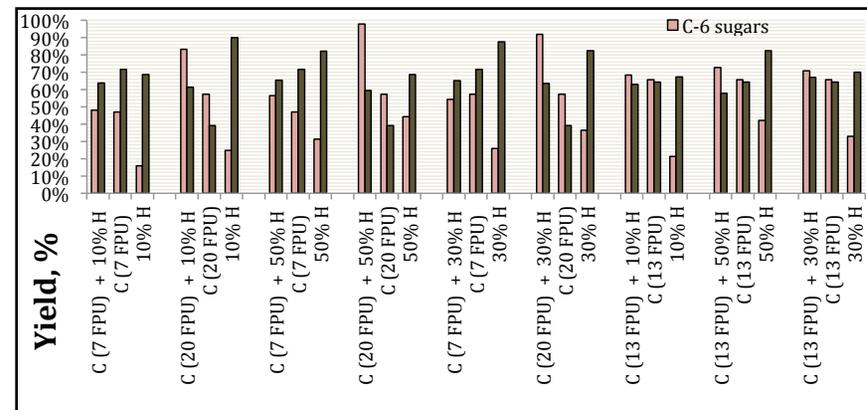
Figure PPB-2. Calculated yield obtained from optimization of enzymatic hydrolysis of FS-01 (Enzyme Loading, C=Cellulase, H=Hemicellulase).
