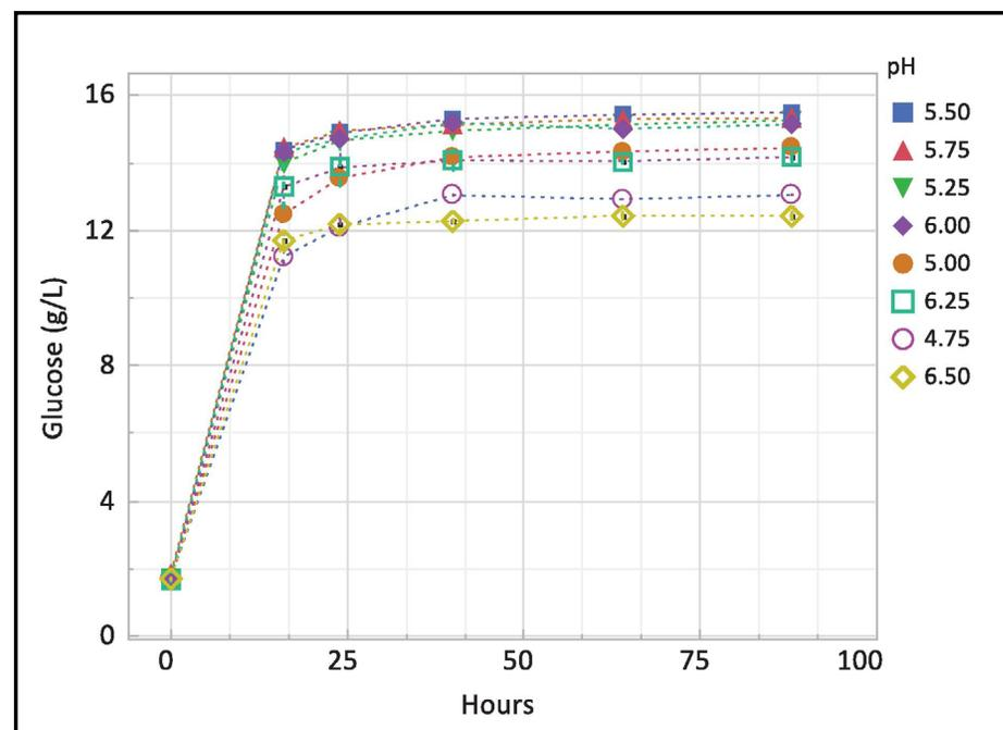
Figure PPB-8. Effects of pH on the hydrolysis of the pretreated sample under optimal pretreatment conditions for maximum cellulose digestibility (190 °C, 7.5% O<sub>2</sub> loading, and 30 minutes residence time).
