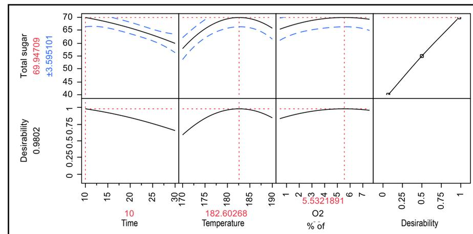
Figure PPB-6. Prediction profiler indicating the pretreatment conditions needed to archive maximum total sugar concentration in the raw pretreatment liquid.
