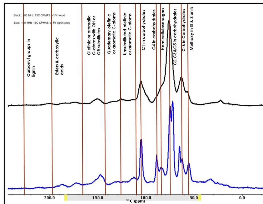
Figure PPB-app.1. Solid-state NMR spectra of untreated FS-10 and biorefinery lignin stream; black line showing  $^{13}\text{C}$  CPMAS spectra at 1MHz for FS-10 and blue line showing  $^{13}\text{C}$  CPMAS spectra at 1MHz for biorefinery lignin.
