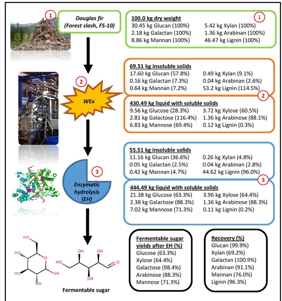
Figure PPB-9. Overall mass balance of the optimal run (190 °C, 7.5% O<sub>2</sub> loading, and 30 minutes residence time).
