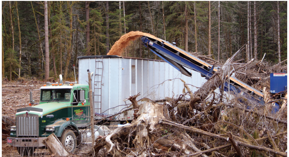
A truck is loaded with chipped residual biomass following timber harvest. The carbon footprint of the operation is smaller when larger trucks are used because fewer trips are needed.
